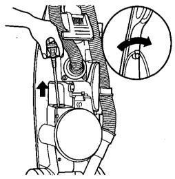
1) To release the power supply cord pull it out by hand and fix it on the power supply cord clip in order to help secure the cord during use.
